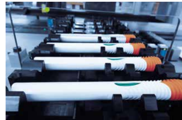
Pen Insertion Pens or Injectors are delivered lying down through a puck system
