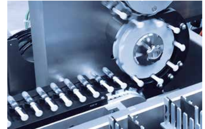
Syringe Infeed With overhead conveyor and no glass on glass contact
