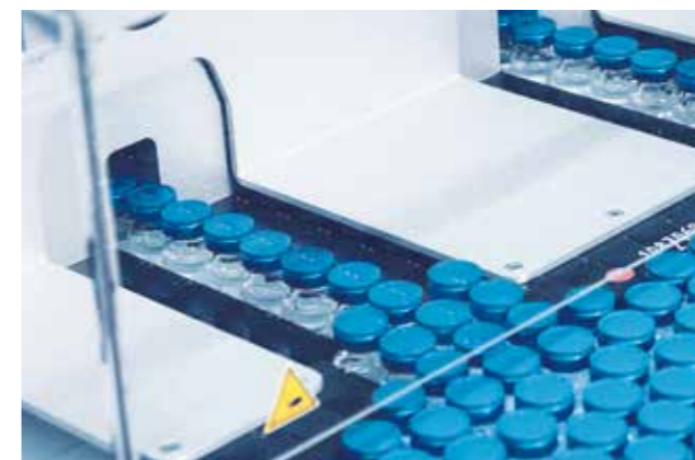
Vial Infeed Standing Vials are delivered via a feeding table to the pick and place handling units
