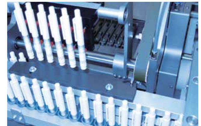
Pen Insertion Pens or Injectors are delivered standing upright through a puck system
