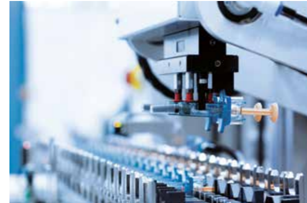
Syringe Inserter The Syringes are delivered lying down through a puck system
